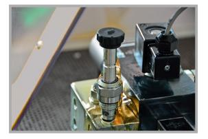
100% of the valves are tested to ensure that internal leakage levels are kept to a minimal amount, less than 5 drops per minute even for the larger sizes of valve.
