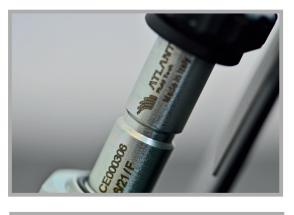
Special tubes have been designed to work reliably at the highest pressures. The employment of non-welded construction and the use of high-strength materials have produced valves that can work at 500 bar (7200 psi) with a burst pressure of 1300 bar (18800 psi).
